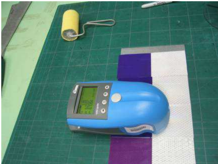
Figure 45. Color measurements Taken with BYK Gardner Instrument.
