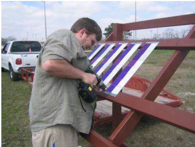
Figure 47. Installation of Panels on Weathering Rack.
