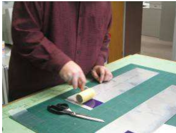
Figure 42. Application of Individual Samples to Weathering Panel.
