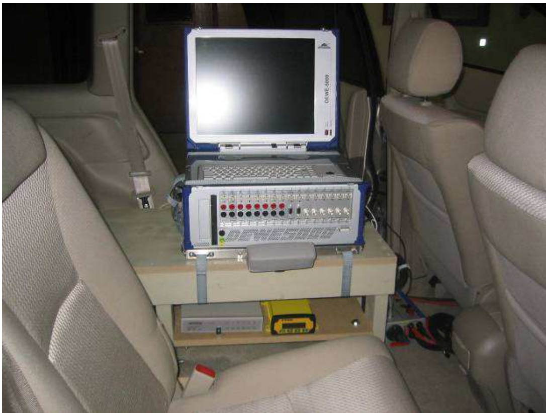
Figure 24. Texas Transportation Institute's Instrumented Vehicle.
